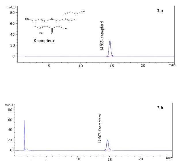
Figure 2: HPLC chromatogram of (a) Std. kaempferol and (b) Isolated kaempferol in mobile phase solution A (water: orthophosphoric acid, pH 3.0) and solution B (acetonitrile: methanol in ratio of 75:25) (50:50) scanned at 370 nm
