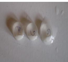
(c) Fig.No.6: Tablets of Atomoxetine HCl at (a) 4 hrs (b) 6 hrs (C) triplicates at 8 hrs of Dissolution.
