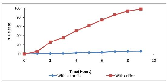
Fig.No. 11: Release profile of formulation with & without delivery orifice
