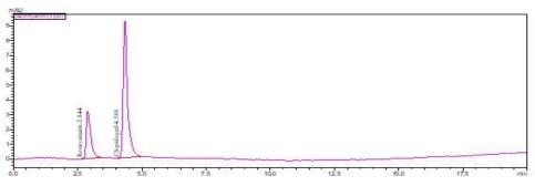
Figure 5: A typical chromatograph of mixture of standard RSV and CLO Rosuvastatin calcium (RSV) and Clopidogrel bisulfate (CLO) with Rt of 2.844 min. and 4.388 min. respectively.
