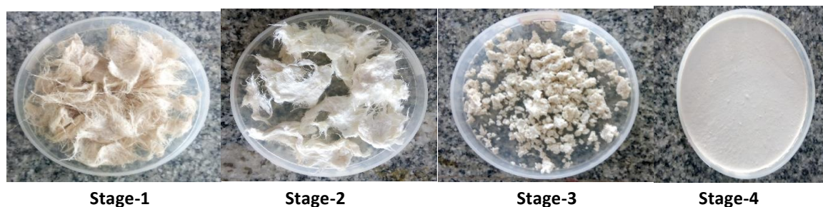
Figure-1: Photograph of steam exploded banana fibers at various stages
