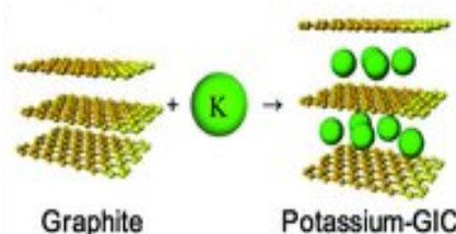
Fig. 2. Graphite Intercalation Compound
