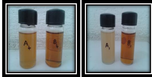
Fig -1: change of colour(Formation of brownish yellow ) due to silver nanoparticle synthesis by methanolic extracts of Heterodermia boryi and Parmotrema stuppeum
