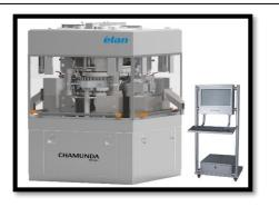
Fig 4: Direct compression machine
