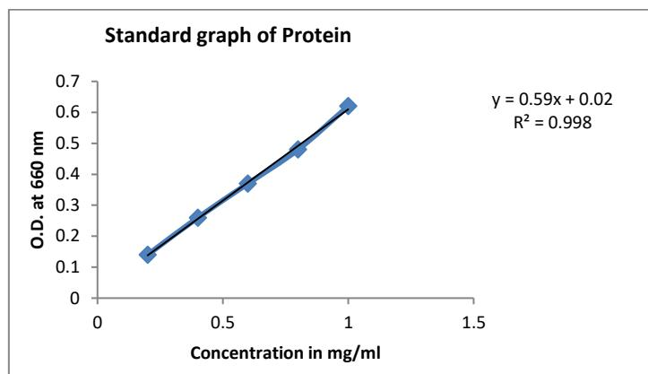
The concentration of all the unknown samples were determined using the equation  $y = 0.59x + 0.02$  which was obtained from the standard graph. The results are tabulated as below:
