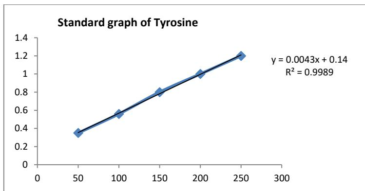
The concentration of all the unknown samples were determined using the equation  $y = 0.004x + 0.14$  which was obtained from the standard graph. The results are tabulated as below
