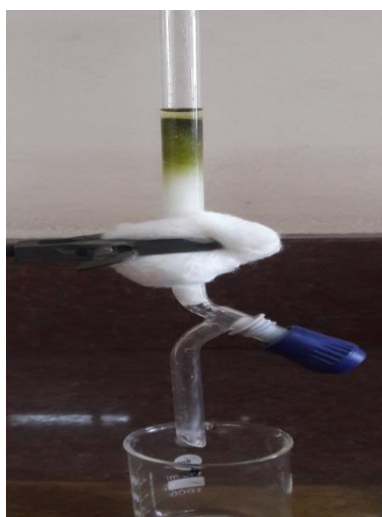
Figure 17: Extraction of parthenin by column chromatography
