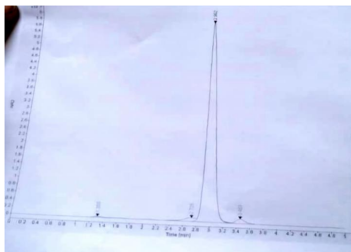
Figure 4: Standard Fipronil Chromatogram
