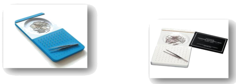
Figure8: 'O'Connor Tweezer Dexterity test instrument
