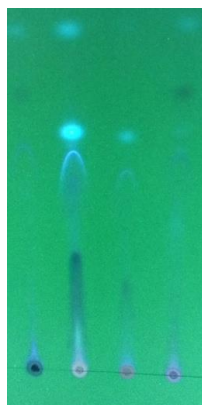
Fig. 5: Chromatogram of methanolic extracts of fungi CRIR 1, CRIR 2, CRIL1 A and CRIL1 B developed by thin-layer chromatography using solvent system ethyl acetate Methanol:Chloroform:Hexane. Dark spots were observed in ultraviolet light against green background confirming the presence of flavonoids
