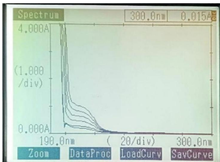
Fig. 4: Spectrum showing overlay of Pregabalin derivative at different concentrations.
