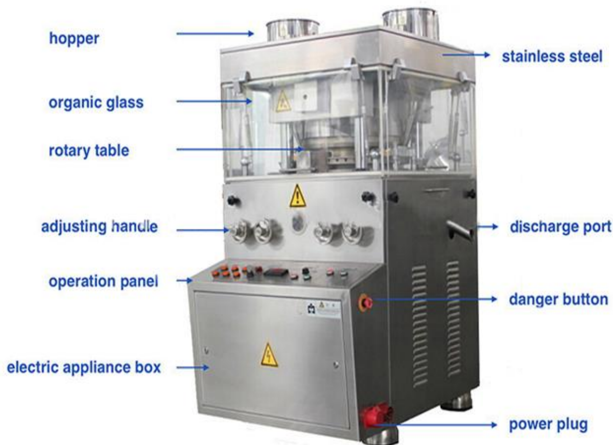
Fig. 1 rotary type tablet punching machine with labeling (www.pharmapproach.com)
