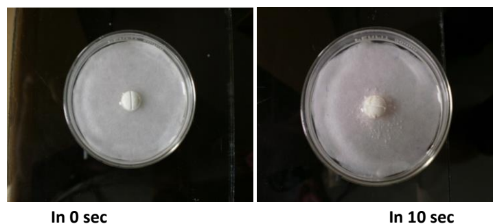
Fig. 6: Diagram showing various steps involved in the disintegration of the tablet
