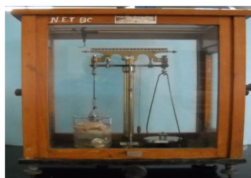
Figure 2: Measurement of ex vivo bioadhesive strength
